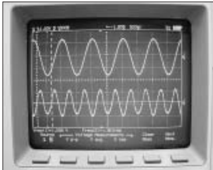
PHOTO 5: 12FM6, 13.5V bias, 1V RMS out (top) and distortion residual (bottom).
