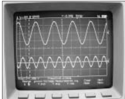
PHOTO 7: 12FM6, 19V bias, 1V RMS out (top) and distortion residual (bottom).
