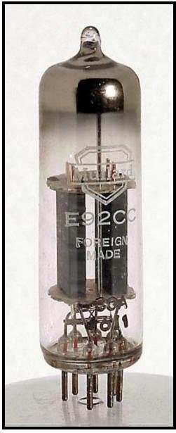
The E92CC double triode is a special quality valve and was designed for use in digital circuits such as flip-flops and counter tube drivers.
